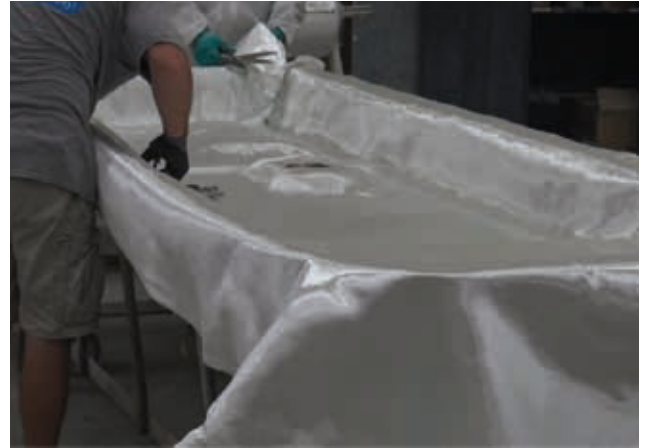
2. Glass fitted and packed.
