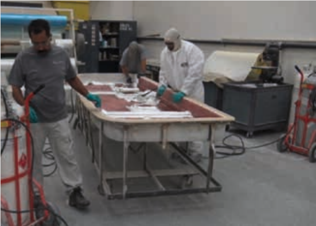
1. Lay-up of the swim platform.
