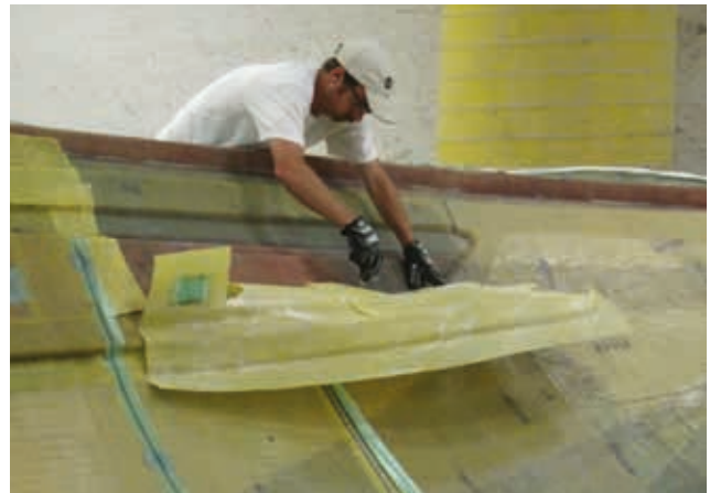
10. Peeling Compoflex® RF 3 is very easy and time-saving.
