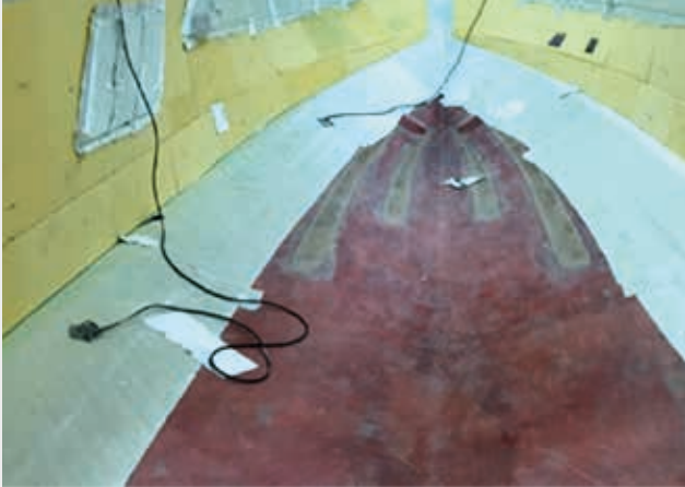
1. Lay-up glass and core.
